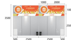
展位侧立面图 Side elevation of booth
