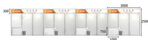
展位正立面图 Front elevation of booth
