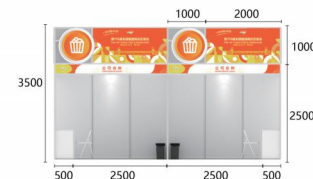
展位侧立面图 Side elevation of booth
