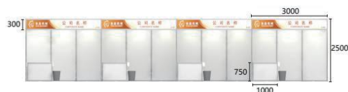
展位正立面图 Front elevation of booth
