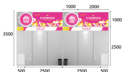
展位侧立面图 Side elevation of booth
